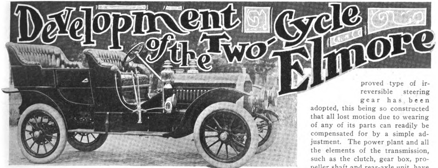
THE ELMORE "40"—THE TWO-CYCLE, FOUR-CYLINDER, "VALVELESS" CAR.
